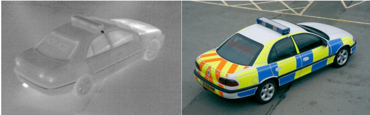
FIGURE 2 Standard retro-reflective livery materials do not show up on thermal camera images
